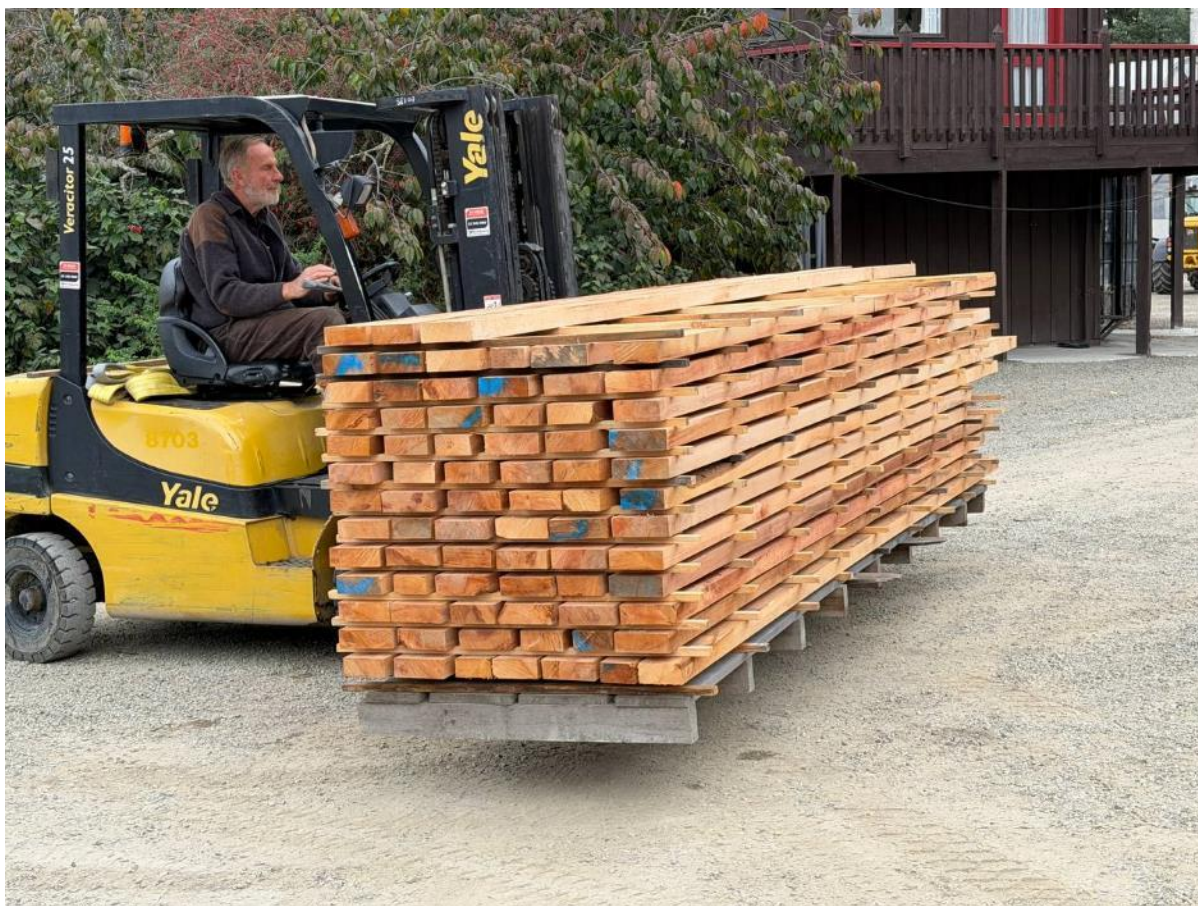
Figure 11 – Some tōtara boards stacked in fillet to air-dry while awaiting repair of the drying kiln at John Fairweather's yard, Specialty Timber Solutions. Photo supplied by Guido Loeffler.
